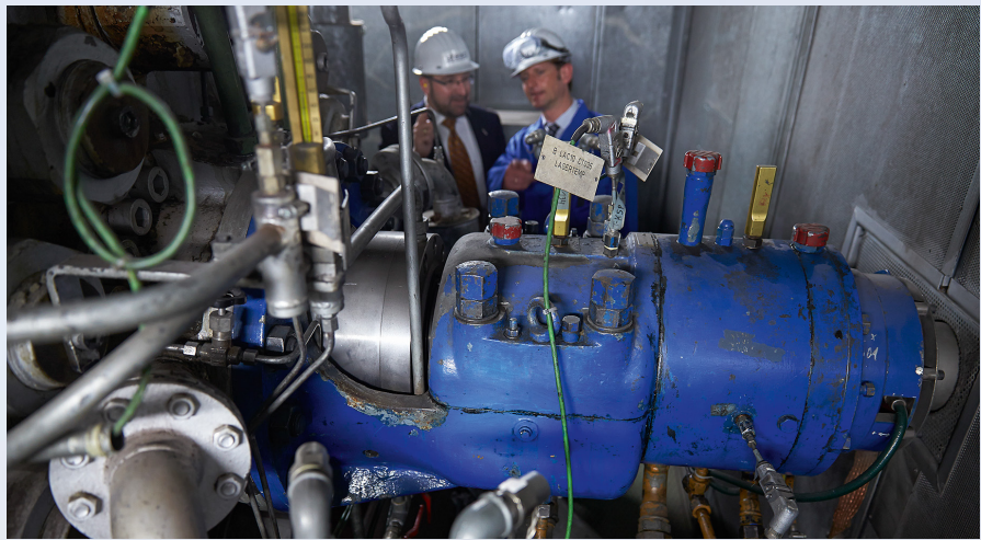
The specialists Andreas Kretschmer and Christoph Bolte are satisfied: The diamond-faced mechanical seal has been operating without problems for more than 13,000 hours.
